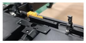
7. Install the front camera and rear tail light; note that you can install the camera/tail light on the fixing seat first, and install it on the cover after paying attention to the wiring;
