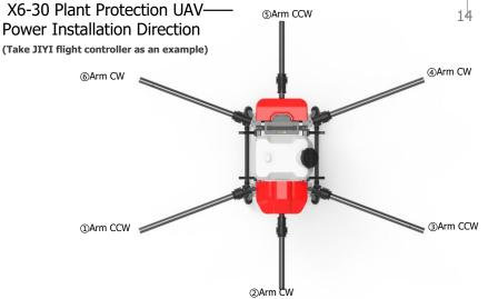
\* The arm steering in the picture is JIYI flight control as an example, and the installation position of the arm of different flight controllers is different;
