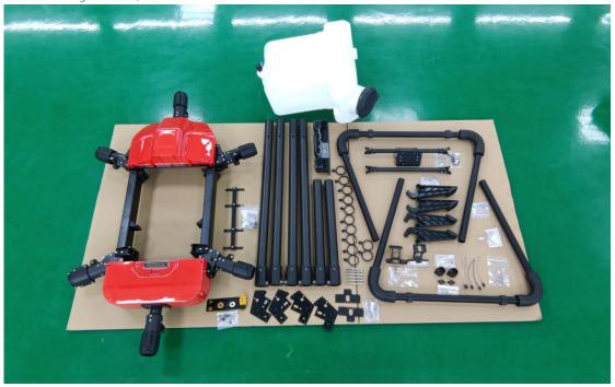
Contents include: frame main body; machine arm; tripod; water tank; distribution board; radar installation kit + tripod rod; water pipe buckle; front camera mount and rear taillight mount; arm buckle; under the arm holder Cover plate; RTK mounting base; remote control antenna mounting base; battery buckle; arm mounting screws; wire
