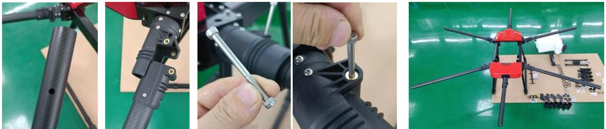
Hole down Sequential installation Install the arm screws M5\*60, The installation is complete as shown above
