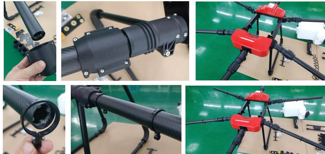
5. The arm is snap-fitted; it is divided into left L and right R, and the nose is lower and the tail is upper;
