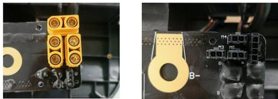
Tail power signal interface, 2P is the power signal output, 4P is the signal extension interface, corresponding to the embedded 4P line, M3, M4, M5 correspond to CH3, CH4, CH5 of the extension line
