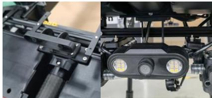
Note: When installing the front camera, fix the camera first, and then install it to the cover plate after the wiring is completed. Before installing the cover plate, you need to confirm the power and after the wiring of other modules is completed, lock it at last
