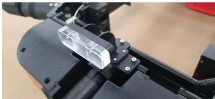
Note: When installing the tail light, fix the tail light first, and then install it to the cover after the wiring is completed. Before installing the cover, you need to confirm the power and other modules. After the wiring is completed, the tail light needs to be extended first, and the tail light is fixed with screws , and finally lock the cover
