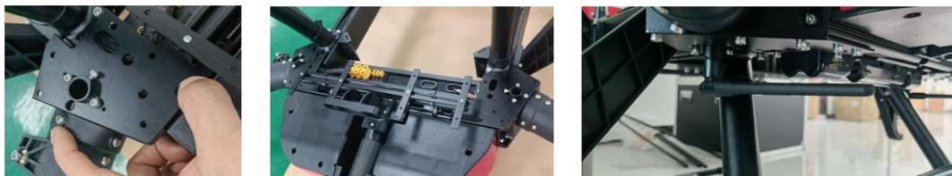
9. RTK fixed base installation; RTK needs to be fixed on the matching mounting base first, then install the antenna connector and lock it on the installation position (M3\*12), note that 3M double-sided tape can be used to fix the RTK antenna, or you can use an optional Fix the glue by curing; lead out the antenna connector end inside the machine head in advance;
