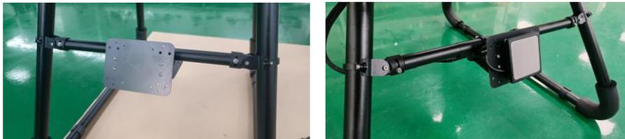
12. GPS installation; there is a special GPS installation position inside the machine head, first remove the GPS installation platform plate, locate the GPS direction and lock it; the schematic diagram of the distribution of modules inside the case;
