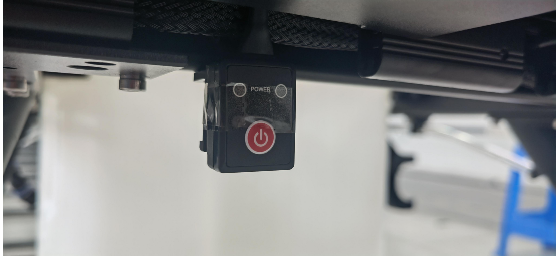
电源电池开关，短按加长按开机，短按加长按关机； Power battery switch, short press the extension button to turn on, short press the extension button to turn off;
